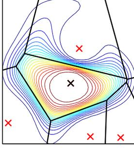
Fig. 1. Probability density  $\psi_i(x)$  (represented by the level curves) for a particular antenna  $i$  (the central black 'X'), showing neighboring antennas (the red 'X's) and the local Voronoi tessellation (in dark lines). The density can be seen as a smoothed Voronoi tessellation, where there is also some (small) probability to be connected to antenna  $i$  when the user is in another Voronoi cell.
